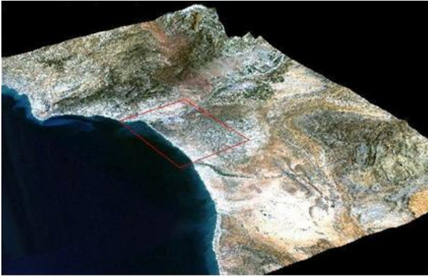
Fig 1: 3D visualization of the RGB composite (TM 3 - TM 2 - TM 1) of the Landsat ETM+ image
