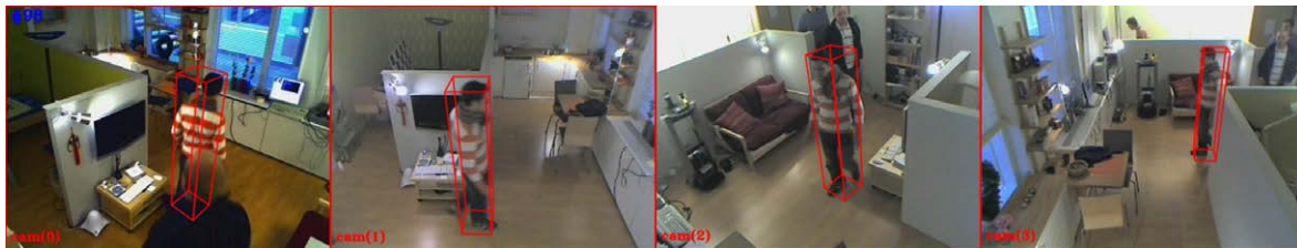
Fig. 3. Projection of the 3D geometric model employed for tracking people. Cameras are calibrated in order to calculate the model projection in each camera.
