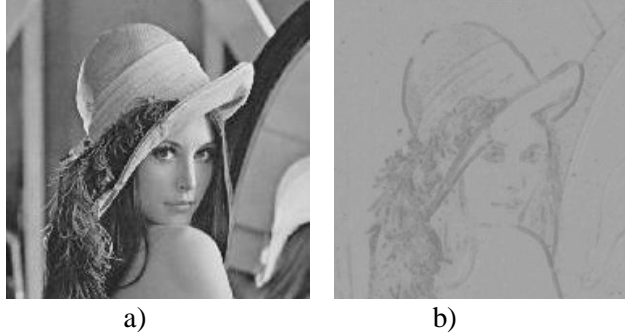
Fig.5.19(II): Applying the neutrosophic top-hat filter: a) Original image b) Neutrosophic top-hat boundary filtered in type II
