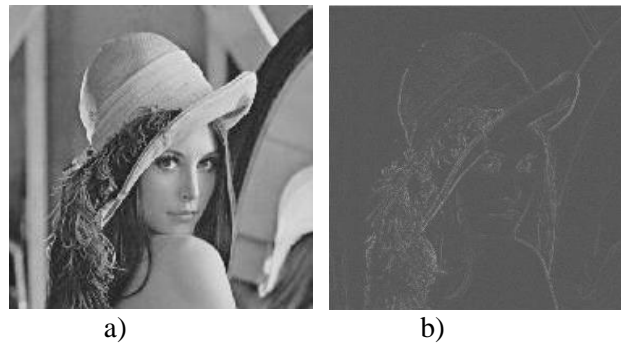
Fig. 5.13(I): Applying the neutrosophic internal boundary: a) Original image b) Neutrosophic internal boundary filtered image
