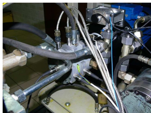
Figure 2. View of the vibration transducers mounted on the body of the tested pump.
