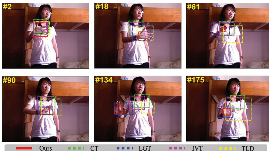
Fig. 4. Screenshots of tracking results of the video sequence used for testing ( hand_no_occ , target is selected in frame #1).
