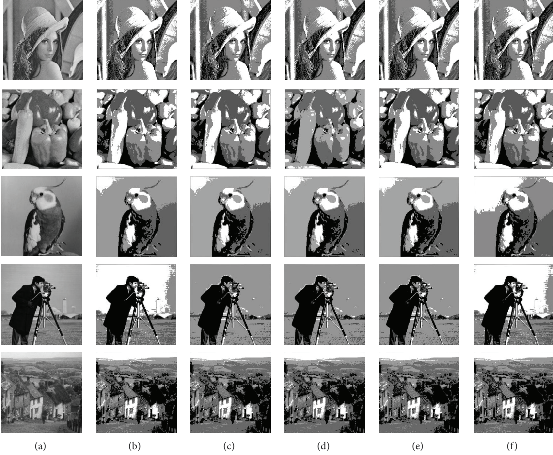
FIGURE 7: Four-level segmentation results of different algorithms: (a) origin image, (b) segmented image using our method, (c) segmented image using BA algorithms, (d) segmented image using MMSA algorithms, (e) segmented image using IBA algorithms, and (f) segmented image using OTSU algorithms.
