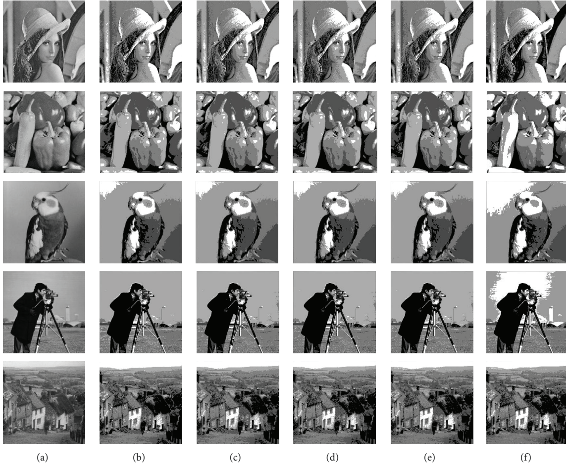
FIGURE 8: Five-level segmentation results of different algorithms: (a) origin image, (b) segmented image using our method, (c) segmented image using BA algorithms, (d) segmented image using MMSA algorithms, (e) segmented image using IBA algorithms, and (f) segmented image using OTSU algorithms.
