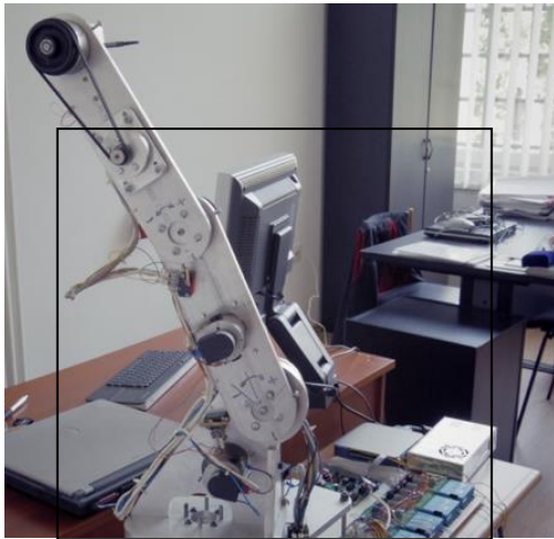
Fig. 2. The didactical arm type robot used in the assisted research.
