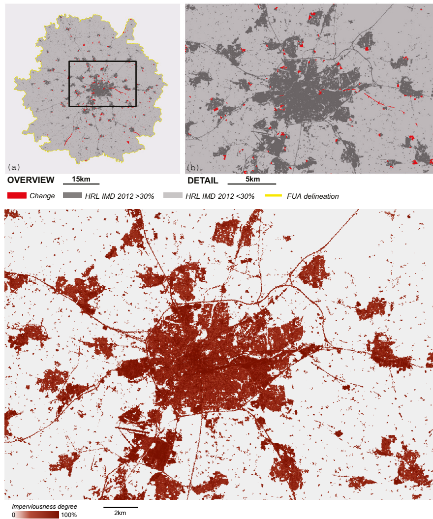
Figure 12. 2012 to 2015 change detection map in Rennes. Changes have been detected by comparison of the Copernicus HRL IMD (in 2012) and our product (in 2015). (a) The entire area; (b) a zoom of the black squared area.
