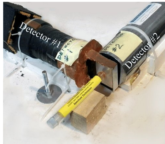
Fig. 2: Two \gamma -ray detectors in tandem geometry; a demonstrator unit. Detector #1 was used with other components for data shown.
