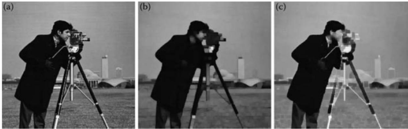
FIGURE 3.5 An example of grayscale morphological operations by a 5 \times 5 square with all 0s: (a) the Cameraman image, (b) the grayscale opening, and (c) the grayscale closing.
