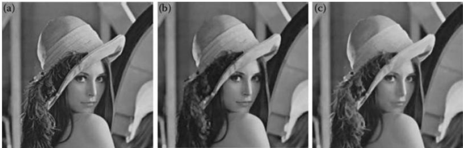
FIGURE 3.4 An example of grayscale morphological operations by a 3 \times 3 square with all 0s: (a) the Lena image, (b) the grayscale opening, and (c) the grayscale closing.
