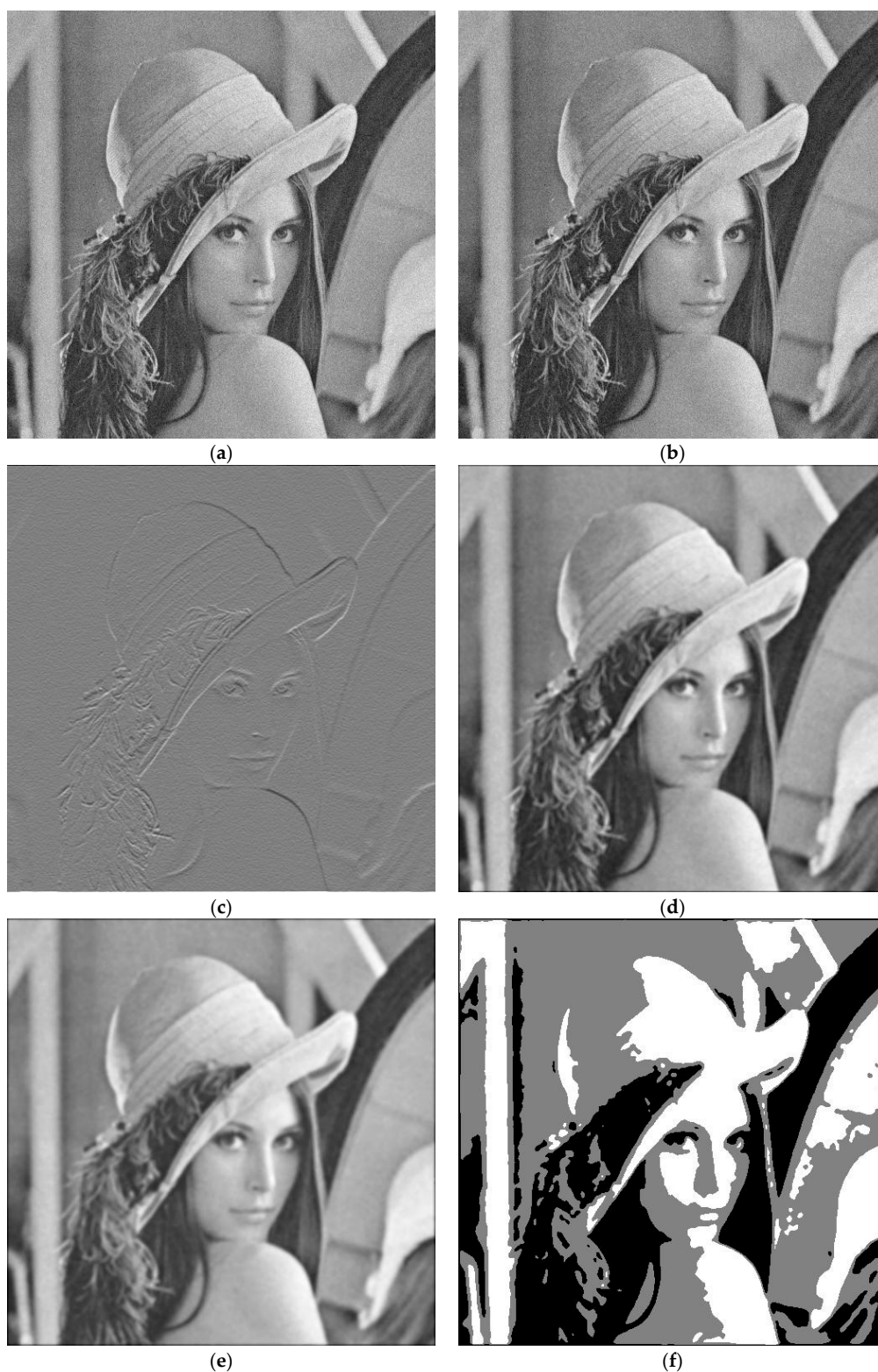
Figure 2. Intermediate results for “Lena” image: (a) Original image; (b) Result of T_s ; (c) Result of I_s ; (d) Filtered result of T_s ; (e) Filter result of T_n ; (f) Final result.
