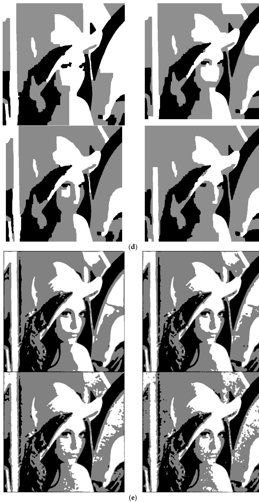
Figure 6. Comparison results on “Lena” image: (a) “Lena” image with different Gaussian noise level: variance: 0, 10, 20, 30; (b) Segmentation results of NSC; (c) Segmentation results of GC; (d) Segmentation results of KGC; (e) Segmentation results of NGC.
