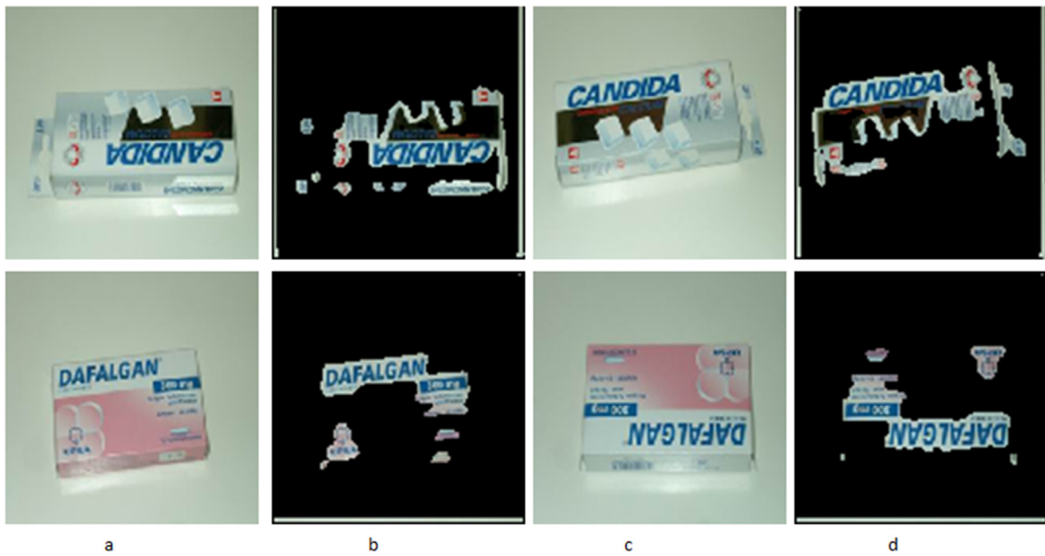
Fig. 12. Column wise (a) Color text image set from Computer vision Laboratory dataset. (b) Text region segmentation results of corresponding images in (a) in the same sequence, using the proposed method. (c) Another set of color text image set corresponding to the same row in (a) with the different orientation. (d) Text region segmentation results of corresponding images in (c) in the same sequence, using the proposed method.
