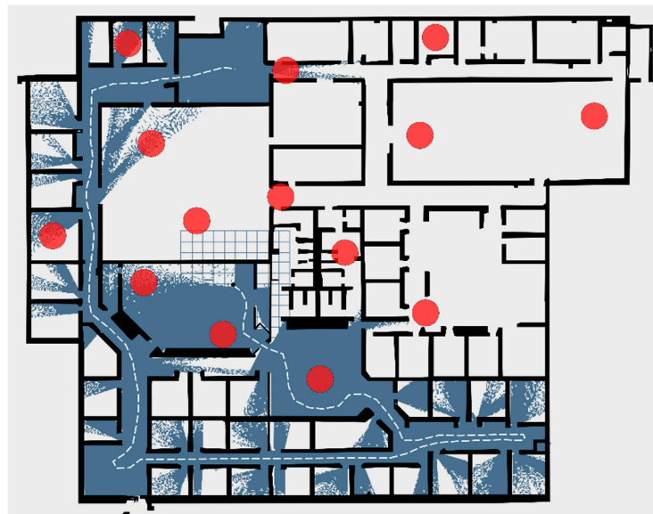
Figure 6. Total scanned area in a 20-minute time interval, using the proposed sustainable exploration strategy. The red dots represent static fire obstacles, that robot must avoid. Robot movement trajectory is coloured in white.
