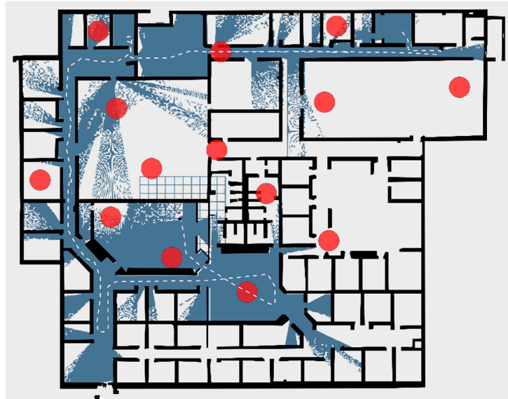
Figure 5. The total scanned area in a 20-minute time interval, using the greedy exploration strategy. The red dots represent static fire obstacles, that robot must avoid. Robot movement trajectory is coloured in white.
