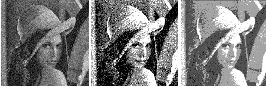
FIGURE 4. For Lena2 image, the first part is the original image with gaussian noise (mean is 0 and variance is 0.01), the middle part is the segmentation by the traditional k -means algorithms, and the third part is the segmentation by interval neutrosophic set method
