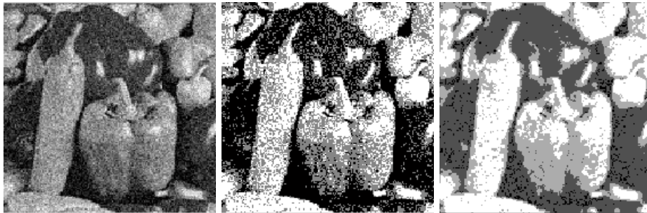
FIGURE 5. For Pepper image, the first part is the original image with gaussian noise (mean is 0 and variance is 0.01), the middle part is the segmentation by the traditional k -means algorithms, and the third part is the segmentation by interval neutrosophic set method
