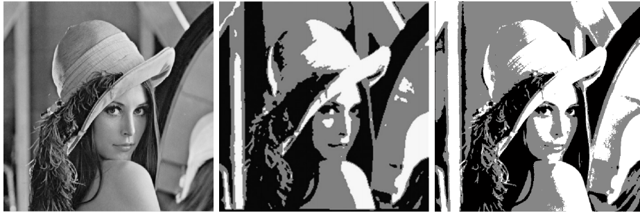
FIGURE 6. For Lena image, the first part is the original image, the middle part is the segmentation by the approach in [9], and the third part is the segmentation by interval neutrosophic set method
