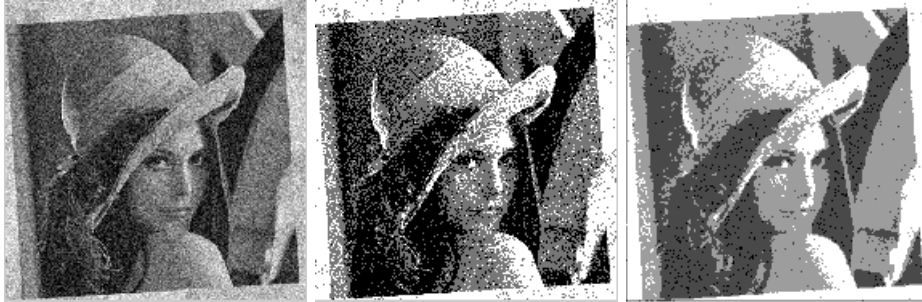
FIGURE 3. For Lena image, the first part is the original image with gaussian noise (mean is 0 and variance is 0.01), the middle part is the segmentation by the traditional k -means algorithms, and the third part is the segmentation by interval neutrosophic set method
