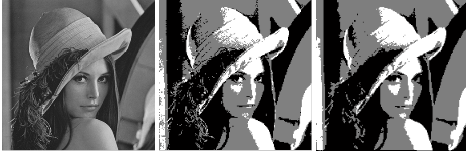
FIGURE 2. The first part is the original image, the middle part is the segmentation by the traditional k -means algorithms, and the third part is the segmentation by interval neutrosophic set method
