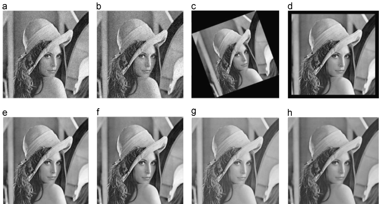
Fig. 7. Attacked watermarked images: (a) Gaussian noise ( M=0 , \text{var}=0.005 ), (b) salt and pepper noise (density=0.001), (c) rotation by 20°, (d) cropping 20 pixels each side, (e) upscale re-size, (f) downscale re-size (g) gamma correction, (0.8) and (h) median filter ( 5 \times 5 ).
