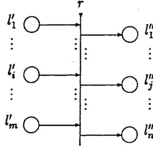
(a)  $L'$  and  $L''$  are finite, non-empty sets of places (the transition's input and output places, respectively); for the above transition these are
