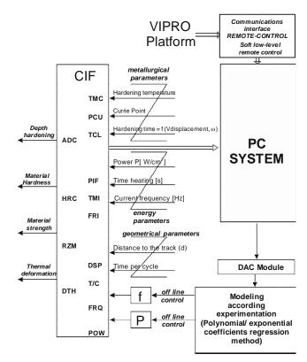
Figure 2: HFC Hardening System Architecture
