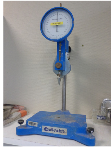
Fig. 13. Laboratory penetration cone.
